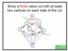
Figure 4. Finding a finite value cut in a graph. In this example, the students were asked to find a finite value (S,T) cut in a graph where the solid (black) edges were all assigned infinite costs. The point was to illustrate the importance of the asymmetry: an infinite cost edge from T to S is not a problem, unlike from S to T.
